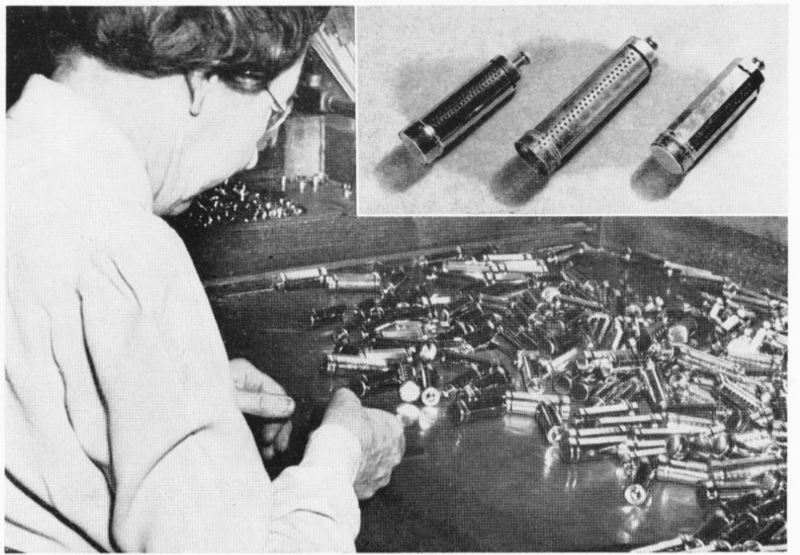
Well qualifying as a Scovill "old-timer" is the dime bank pictured above. It has been a product of the Main Plant for almost sixty years — records show dime banks (left and right, insert) and penny banks were made here back in 1890. Above, today's banks are assembled, inspected and packed for shipment in the Assembly Room. Ann Wheelaban is the operator.
